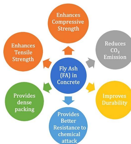
Figure 1. key benefits of incorporating Fly Ash (FA) in concrete, highlighting its role in enhancing strength, durability and sustainability.
