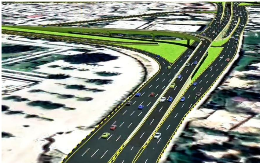
Figure 9: Proposed geometric redesign and traffic improvement scenario for T-Chowk intersection
