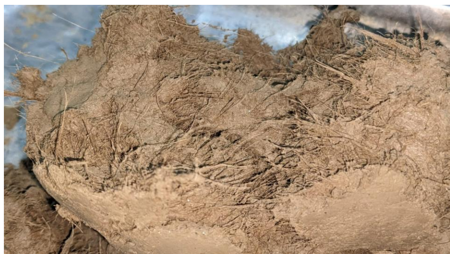
Figure Error! No text of specified style in document.-2 Soil Mixed with Sisal Fiber
