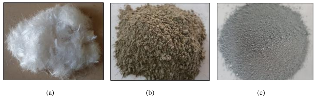
Figure 1. Material (a) Polypropylene fibers (b) Bentonite (c) Silica fume
