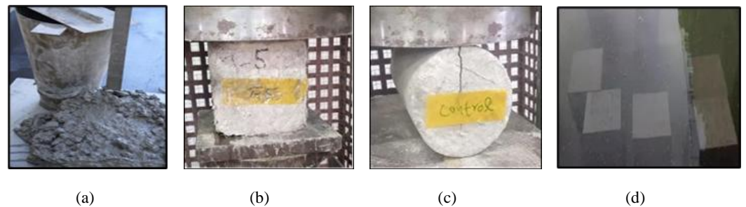
Figure 2. (a) Workability, (b) Compressive Strength Test, (c) Split Tensile Strength Test, (d) Water Absorption Test
