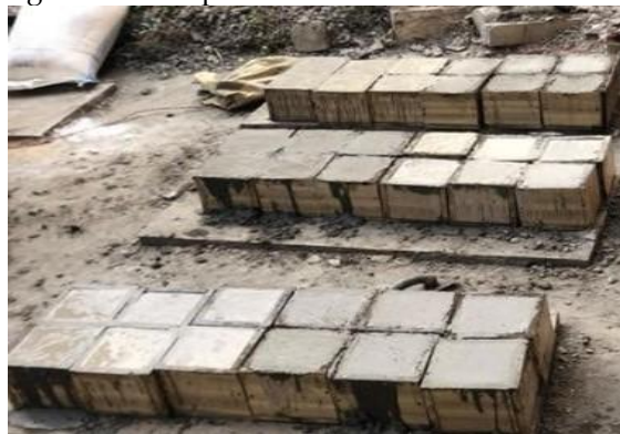
Figure 1. Concrete cube moulds sample preparation.
